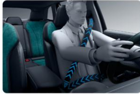
Active preload seat belt
