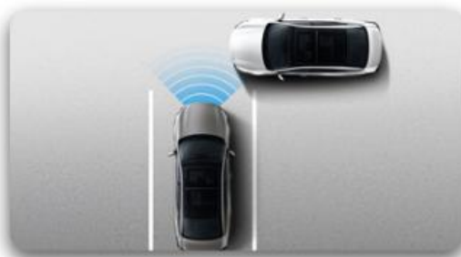
▲ MOD Moving object/pedestrian alert
