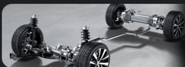
AMVAR variable Independent suspension & five link independent suspension
