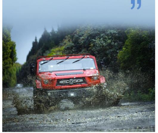
The car's approach angle is 45 degree, departure angle is 35degree, the minimum ground clearance is 380mm, which allows the car to complete 60 degrees of climbing. And the height of 2.3 meters also allows it to have amazing wading ability, the original state can reach 0.75 meters of wading depth.
