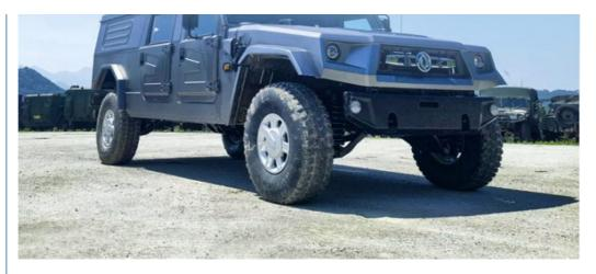
Dongfeng Mengshi M50 has high maneuverability, high passability and high reliability. Max speed 120km/h, max driving range 600km, max climbing height over 60%, max vertical obstacle crossing more than 400mm, max Wading Depth 1.2m. It can be driven about 4500m above sea in low temperature
