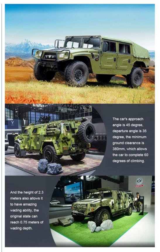
The car's approachangle is 45 degree, departure angle is 35 degree, the minimum ground clearance is 380 mm, which allows the car to complete 60 degrees of climbing.
