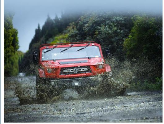
The car's approach angle is 45 degree, departure angle is 35degree, the minimum ground clearance is 380mm, which allows the car to complete 60 degrees of climbing. And the height of 2.3 meters also allows it to have amazing wading ability, the original state can reach 0.75 meters of wading depth.
