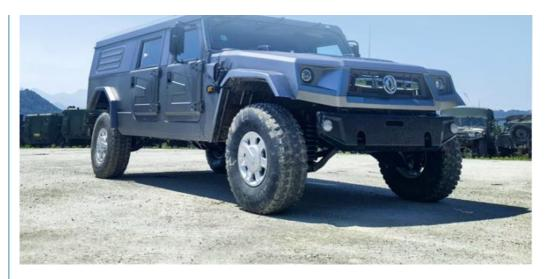
Dongfeng Mengshi M50 has high maneuverability, high passability and high reliability. Max speed 120km/h, max driving range 600km, max climbing height over 60%, max vertical obstacle crossing more than 400mm, max Wading Depth 1.2m. It can be driven about 4500m above sea in low temperature
